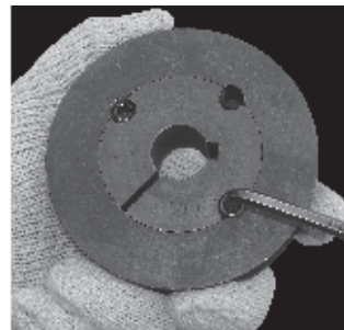
Step 4: Tighten them further using allen-key. Tighten the screws alternately
