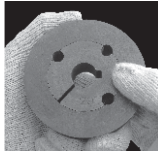
Step 2: Match the holes of pulleys with those of the bush
